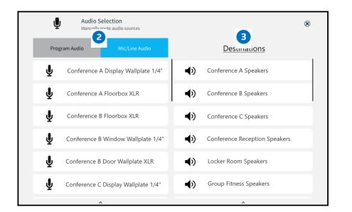
1 From the Home Screen, Select Audio Routing for advanced routing control allowing multiple sources to route to multiple rooms
